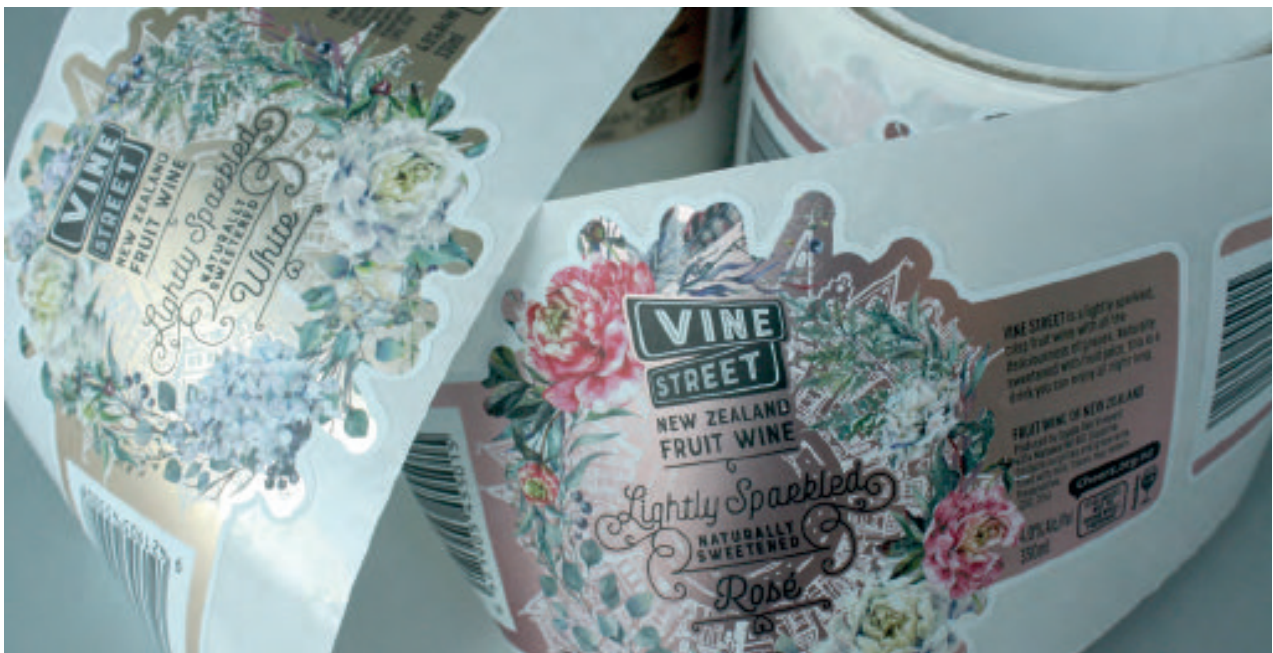
New Zealand's Soar Print won a World Label Award for its Vine Street wine labels, using Manta OPP silver metallised substrate, printed on an HP Indigo WS6800, and sealed with a matte laminate before die-cutting
